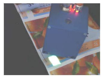
Detecting front and back side of a metal strip
